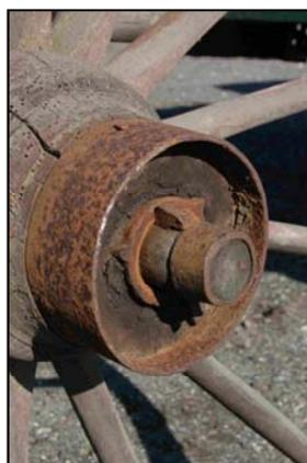
*Close-up of axle showing Lynch Pin (a simple vertical pin through axle) holding wheel on axle.*
