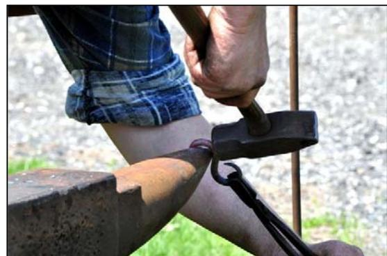
*At a Plow Day demonstration, blacksmith Tim Greene is fabricating a figure 8 link to connect chain.*
