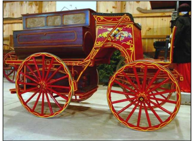
*Skyline Farm's unique piano moving wagon is sprung specifically for that purpose. A rare cylinder player piano is loaded aboard to illustrate how it's mounted on the vehicle.*
